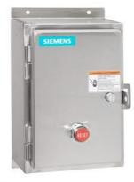
Non-reversing motor starter Size 4 Three phase full voltage Solid-state overload relay OLRelay amp range 50-200A 220-240/440-480VAC 60HZ coil Combination type Water/dust tight non-corrosive
