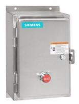
Non-reversing motor starter, Size 4, Three phase full voltage, Solid-state overload relay, OLR amp range 50-200A, Non-combination type, Encl. type 4X 304 S. Steel, Water/dust tight noncorrosive, Standard width enclosure
