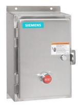
Non-reversing motor starter, Size 4, Three phase full voltage, Solid-state overload relay, OLR amp range 50-200A, 24VAC 50-60Hz coil, Non-combination type, Encl. type 4X 304 S. Steel, Water/dust tight noncorrosive, Standard width enclosure
