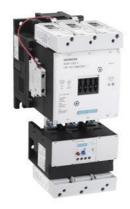
Non-reversing motor starter Size 6 Three phase full voltage Solid-state overload relay OLRelay amp range 160-630A 200-220V 50-60HZ/DC coil Combination type No enclosure
