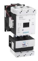
Non-reversing motor starter Size 6 Three phase full voltage Solid-state overload relay OLRelay amp range 160-630A 23-26V 50-60HZ/DC coil Combination type No enclosure
