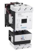
Non-reversing motor starter Size 6 Three phase full voltage Solid-state overload relay OLRelay amp range 160-630A 240-277V 50-60HZ/DC coil Combination type No enclosure
