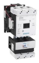
Non-reversing motor starter, Size 8, Three phase full voltage, Solid-state overload relay, OLRelay amp range 400-1200A, 100-250V 50-60HZ/DC coil Noncombination type, Enclosure type (open), No enclosure
