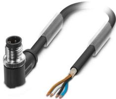
Sensor/actuator cable, 4-position, PUR halogen-free, black-gray RAL 7021, shielded (Tinned copper braided shield), Advanced Shielding Technology, Plug angled M12, coding: A, on free cable end, cable length: 10 m
