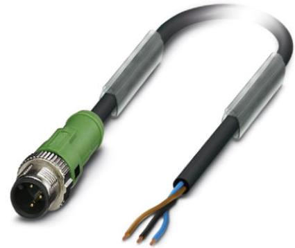
Sensor/Actuator cable, 3-position, PUR, halogen-free, Black-gray RAL 7021, Plug, straight M12-SPEEDCON, A-coded, on Free conductor end, Cable length: 3 m
