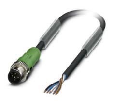
Sensor/Actuator cable, 5-position, PUR, halogen-free, Black-gray RAL 7021, Plug, straight M12-SPEEDCON, A-coded, on Free conductor end, Cable length: 3 m
