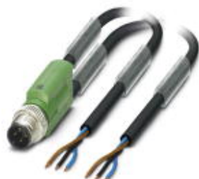
Sensor/actuator cable, 3-position, PUR halogen-free, black-gray RAL 7021, Plug straight M12 SPEEDCON, A-coded, on free cable end and free cable end, cable length: 5 m
