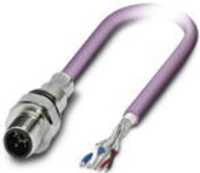
Bus system flush-type plug, DeviceNet/CANopen, 5-pos., M12, shielded, A-coded, front/screw mounting with M16 thread, with 0.5 m bus cable, 2 x 0.2 mm², 2 x 0.32 mm²
