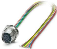
Device connector, rear mounting, Universal, 8-position, Socket, straight, M12-SPEEDCON, coding: A, on free cable end, Rear mounting, Pg9, Individual wires, cable length: 0.5 m, 0.25 mm<sup>2</sup>, TPE litz wire, Alternative product in accordance with RoHS II without Exemption 6c (Pb <0.1%) item no.: 1239959
