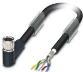
Bus system cable, INTERBUS, 4-position, PUR halogen-free, black RAL 9005, shielded, free cable end, on Socket angled M8, cable length: 20 m
