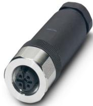
Connector, Universal, 4-position, Socket straight M12, coding: A, Screw connection, knurl material: Stainless steel 1.4404, cable gland Pg9, external cable diameter 6 mm ... 8 mm
