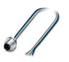
Device connector front mounting, Universal, 4-position, Pin, straight, M12-Standard, coding: A, on free cable end, Front mounting, Pg9, Individual wires, cable length: 0.5 m, 0.34 mm<sup>2</sup>, TPE litz wire
