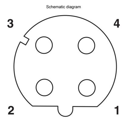
Pin assignment M12 socket, 4-pos., D-coded, female side
