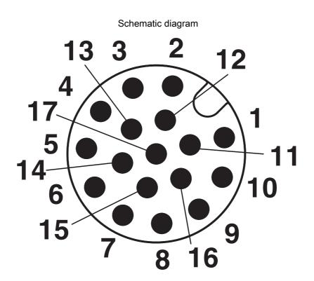
Pin assignment M12 male connector, 17-pos., male side view
