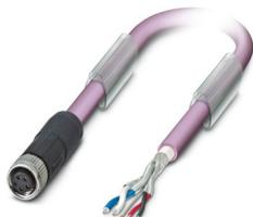
Bus system cable, CANopen®, DeviceNet™, 5-position, PUR halogen-free, red lilac RAL 4001, shielded, free cable end, on Socket straight M8, coding: A, cable length: 5 m, Connector unshielded
