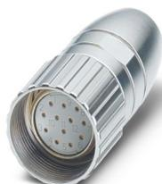
M23, Cable connector, straight, shielded: no, Screw locking mechanism, No. of pos.: 8+1, Direction of rotation: Standard, contact connection type: Socket, Solder cup, cable diameter range: 6.5 mm ... 7.5 mm, coding: N, Alternative product in accordance with RoHS II without Exemption 6c (Pb < 0.1 %) item no.: 1240662
