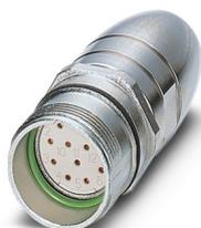
M23, Coupler connector, series: RC, straight, shielded: yes, Screw locking mechanism, No. of pos.: 12, Direction of rotation: Standard, contact connection type: Socket, Solder cup, cable diameter range: 7.5 mm ... 9.5 mm, coding: N, Alternative product in accordance with RoHS II without Exemption 6c (Pb < 0.1 %) item no.: 1241004
