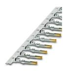
Crimp contact, Socket, rolled, Taped product, number of pieces per reel: 500, contact diameter: 1 mm, crimp range: 0.08  $\rm mm^2$  ... 0.22  $\rm mm^2$
