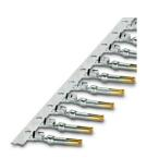
Crimp contact, Socket, rolled, Taped product, number of pieces per reel: 500, contact diameter: 1 mm, crimp range:  $0.22~\text{mm}^2$  ...  $0.56~\text{mm}^2$ , Item is lead-free in accordance with RoHS II without Exemption 6c (Pb < 0.1~%)
