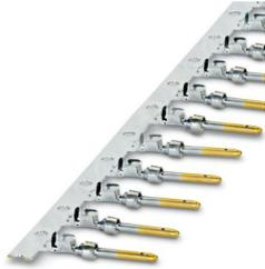
Crimp contact, Pin, rolled, Taped product, number of pieces per reel: 10000, contact diameter: 1 mm, crimp range: 0.08 mm<sup>2</sup> ... 0.22 mm<sup>2</sup>
