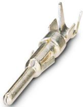
Crimp contact, Pin, rolled, Single contact, contact diameter: 1 mm, crimp range: 0.22 mm<sup>2</sup> ... 0.56 mm<sup>2</sup>, Single contact, Item is lead-free in accordance with RoHS II without Exemption 6c (Pb < 0.1 %)
