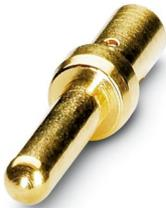
Crimp contact, Pin, turned, Single contact, contact diameter: 1 mm, crimp range: 0.08 mm<sup>2</sup> ... 0.22 mm<sup>2</sup>, Contact release tool not necessary for the 12- and 17-pos. crimp versions of the M23-PRO series, Alternative product in accordance with RoHS II without Exemption 6c (Pb < 0.1 %) item no.: 1240882
