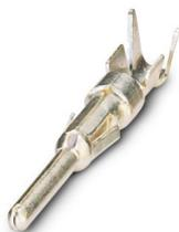
Crimp contact, Pin, rolled, Single contact, contact diameter: 1 mm, crimp range: 0.08 mm<sup>2</sup> ... 0.22 mm<sup>2</sup>, Single contact
