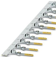
Crimp contact, Pin, rolled, Taped product, number of pieces per reel: 10000, contact diameter: 1 mm, crimp range: 0.22 mm<sup>2</sup> ... 0.56 mm<sup>2</sup>, Item is lead-free in accordance with RoHS II without Exemption 6c (Pb < 0.1 %)
