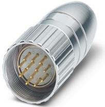
M23, Cable connector, straight, shielded: no, Screw locking mechanism, No. of pos.: 17, Direction of rotation: Standard, contact connection type: Pin, Crimp connection, cable diameter range: 7.5 mm ... 9.5 mm, coding: N
