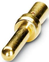
Crimp contact, Pin, turned, Single contact, contact diameter: 1 mm, crimp range: 0.14 mm<sup>2</sup> ... 0.56 mm<sup>2</sup>, Contact release tool not necessary for the 12- and 17-pos. crimp versions of the M23-PRO series, Alternative product in accordance with RoHS II without Exemption 6c (Pb < 0.1 %) item no.: 1240882
