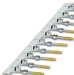
Crimp contact, Pin, rolled, Taped product, number of pieces per reel: 500, contact diameter: 1 mm, crimp range: 0.08 mm<sup>2</sup> ... 0.22 mm<sup>2</sup>
