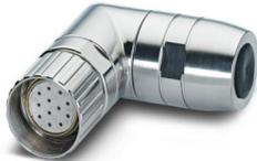
M23, Cable connector, series: UC, angled, shielded: yes, Screw locking mechanism, No. of pos.: 6, Direction of rotation: Standard, contact connection type: Socket, Solder cup, coding: N, Alternative product in accordance with RoHS II without Exemption 6c (Pb < 0.1 %) item no.: 1242078
