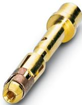
Crimp contact, Socket, turned, Single contact, contact diameter: 1 mm, crimp range: 0.25 mm<sup>2</sup> ... 1 mm<sup>2</sup>, Alternative product in accordance with RoHS II without Exemption 6c (Pb < 0.1 %) item no.: 1241922
