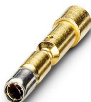
Crimp contact, Socket, turned, Single contact, contact diameter: 1 mm, crimp range: 0.14 mm<sup>2</sup> ... 1 mm<sup>2</sup>, Alternative product in accordance with RoHS II without Exemption 6c (Pb < 0.1 %) item no.: 1241922
