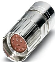
Cable connector, straight, Screw locking mechanism, M23, number of positions: 17, contact connection type: Socket, shielded: yes, degree of protection: IP67, cable diameter range: 6 mm .. 10 mm, number of positions: 17, connection method: Crimp connection, series: RF, Alternative product in accordance with RoHS II without Exemption 6c (Pb < 0.1 %) item no.: 1242282
