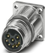
Device connector front mounting, straight, for standard and SPEEDCON interlock, M17, number of positions: 8, contact connection type: Pin, Axial O-ring, 4x Ø2,7, shielded: yes, flange dimensions: 21.6 mm x 21.6 mm, degree of protection: IP67, number of positions: 8, connection method: Crimp connection, series: ST
