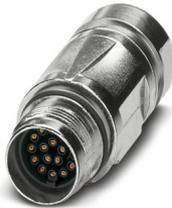
Coupler connector, straight, for standard and SPEEDCON interlock, M17, number of positions: 8, contact connection type: Socket, shielded: yes, degree of protection: IP67, cable diameter range: 8 mm ... 10 mm, number of positions: 8, connection method: Crimp connection, series: ST, Alternative product in accordance with RoHS II without Exemption 6c (Pb < 0.1 %) item no.: 1243385
