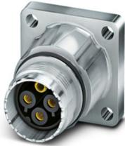
Device connector front mounting, straight, for standard and SPEEDCON interlock, M17, number of positions: 3+PE, contact connection type: Socket, Axial O-ring, 4x Ø 3.2, shielded: yes, flange dimensions: 25.75 mm x 25.75 mm, degree of protection: IP67, number of positions: 4, connection method: Crimp connection, series: ST
