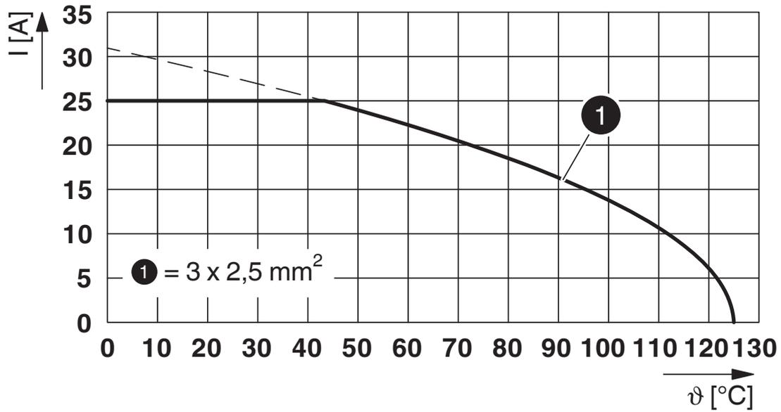
$I$  = current strength,  $\vartheta$  = ambient temperature, 3x 25 A
