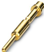
Crimp contact, Pin, turned, Single contact, contact diameter: 1 mm, crimp range: 0.25 mm<sup>2</sup> ... 1 mm<sup>2</sup>, Alternative product in accordance with RoHS II without Exemption 6c (Pb < 0.1 %) item no.: 1241921
