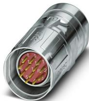
M23, Cable connector, series: CA, straight, shielded: yes, SPEEDCON, No. of pos.: 12, Direction of rotation: Counter direction, contact connection type: Pin, Crimp connection, cable diameter range: 6 mm ... 10 mm, coding: N, Alternative product in accordance with RoHS II without Exemption 6c (Pb < 0.1 %) item no.: 1243579
