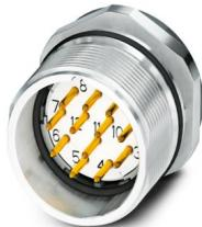
M23, Device connector front mounting, series: CA, straight, shielded: yes, for standard and SPEEDCON interlock, No. of pos.: 17, Direction of rotation: Standard, contact connection type: Pin, Solder connection, Axial seal, Central fastening M20 x 1.5, coding: N, Alternative product in accordance with RoHS II without Exemption 6c (Pb < 0.1 %) item no.: 1243857
