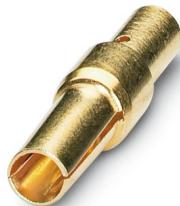
Crimp contact, Socket, turned, contact diameter: 2 mm, crimp range: 1.5 mm<sup>2</sup> ... 2.5 mm<sup>2</sup>, Alternative product in accordance with RoHS II without Exemption 6c (Pb < 0.1 %) item no.: 1241635
