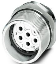
M23, Device connector front mounting, series: CA, straight, shielded: yes, for standard and SPEEDCON interlock, No. of pos.: 7, Direction of rotation: Standard, contact connection type: Socket, Crimp connection, Axial seal, Central fastening Pg13,5, coding: N
