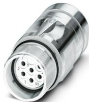
M23, Coupler connector, series: CA, straight, shielded: yes, for standard and SPEEDCON interlock, No. of pos.: 8+1, Direction of rotation: Standard, contact connection type: Socket, Solder connection, cable diameter range: 6 mm ... 10 mm, coding: N, Alternative product in accordance with RoHS II without Exemption 6c (Pb < 0.1 %) item no.: 1244001
