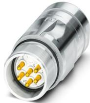
M23, Coupler connector, series: CA, straight, shielded: yes, for standard and SPEEDCON interlock, No. of pos.: 6, Direction of rotation: Standard, contact connection type: Pin, Crimp connection, cable diameter range: 3 mm ... 14.5 mm, coding: N, Alternative product in accordance with RoHS II without Exemption 6c (Pb < 0.1 %) item no.: 1244058
