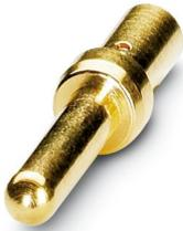
Crimp contact, Pin, turned, contact diameter: 2 mm, crimp range: 1 mm<sup>2</sup> ... 1.5 mm<sup>2</sup>, Alternative product in accordance with RoHS II without Exemption 6c (Pb < 0.1 %) item no.: 1241634
