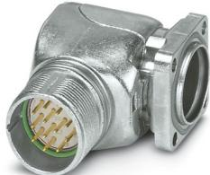
M23, Device connector front mounting, series: RC, angled rotatable, shielded: yes, for standard and SPEEDCON interlock, No. of pos.: 12, Direction of rotation: Standard, contact connection type: Pin, Solder connection, Axial O-ring, 4x Ø 3.2, coding: N, Alternative product in accordance with RoHS II without Exemption 6c (Pb < 0.1 %) item no.: 1244475
