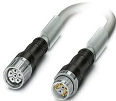
Connector in molded plastic on both sides, series: KSF, M23-Socket, Straight, plastic molded, number of positions: 3+PE, type of locking: Screw locking mechanism, on M23-Pin, Straight, plastic molded, number of positions: 3+PE, cable length: 2 m, shielded: yes, color of outer sheath: gray RAL 7001
