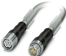
Connector in molded plastic on both sides, series: KSF, M23-Socket, Straight, plastic molded, number of positions: 4+PE, type of locking: Screw locking mechanism, on M23-Pin, Straight, plastic molded, number of positions: 4+PE, cable length: 2 m, shielded: no, color of outer sheath: gray RAL 7001
