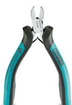
Electronic diagonal cutter, round head, without chamfer, with opening spring, mirror-polished and oiled, 2-component grip, cutting capacity: soft 0.2 - 2.0 mm; medium hard 1.2 mm; hard 0.5 mm diameter
