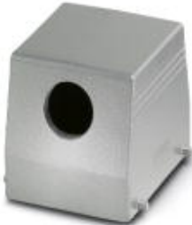
HEAVYCON sleeve housing B32, for double locking latch, height 80 mm, without support 1x M40, lateral conductor exit
