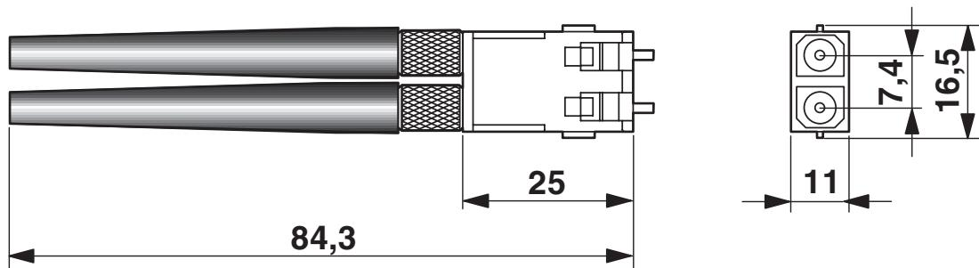
SC-RJ connector, POD, IP20
