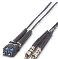
Assembled FO cable, break-out cable, polymer fiber 980/1000 µm, SC-RJ/IP20 on FSMA/IP20, for installation inside the control cabinets, the conductor is suitable for the UV-protected outside insert, length: 2 m
