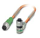
Sensor/actuator cable, 5-position, PUR halogen-free, irradiated, orange RAL 2003, Plug straight M12, coding: A, with 3 LEDs, on Socket angled M12, coding: A, with 3 LEDs, cable length: 1.5 m, Customer-specific version
