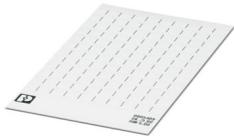
Marker card, Sheet, white, unlabeled, can be labeled with: Marker pen: without print, mounting type: adhesive, for terminal block width: 5 mm, lettering field size: 5 x 3.8 mm, Number of individual labels: 120
