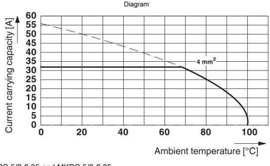
Type: MKDS 5/2-6,35 and MKDS 5/3-6,35 Test following DIN EN 60512-5-2:2003-01 Reduction factor = 1 No. of positions: 5
