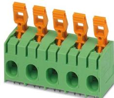
PCB terminal block, nominal current: 76 A, rated voltage (III/2): 1000 V, nominal cross section: 16 mm<sup>2</sup>, number of potentials: 3, number of rows: 1, number of positions per row: 3, product range: PLH 16/, pitch: 15 mm, connection method: Push-lock spring connection, mounting: Wave soldering, conductor/PCB connection direction: 0 °, Pin layout: Linear double pinning, Solder pin [P]: 4.5 mm, number of solder pins per potential: 4, type of packaging: packed in cardboard
