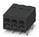
PCB terminal block, nominal current: 6 A, rated voltage (III/2): 160 V, nominal cross section: 0.5 mm², number of potentials: 2, number of rows: 1, number of positions per row: 2, product range: PTSM 0,5/..-H-THR, pitch: 2.5 mm, connection method: Push-in spring connection, mounting: THR soldering, conductor/PCB connection direction: 0 °, color: black, Pin layout: Linear pinning, Solder pin [P]: 2.1 mm, number of solder pins per potential: 2, type of packaging: 24 mm wide tane
