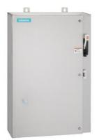
Non-reversing motor starter, Size 3, Three phase full voltage, Solid-state overload relay, OLR amp range 25-100A, 110V 50Hz / 120V 60Hz coil, Combination type, 100A non-fusible disconnect, Encl NEMA type 4X 304 S-Steel, Water/dust tight noncorrosive, Extra-wide enclosure
