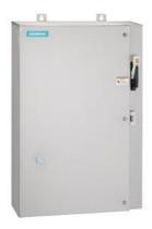
Non-reversing motor starter, Size 3, Three phase full voltage, Solid-state overload relay, OLR amp range 25-100A, 110V 50Hz / 120V 60Hz coil, Combination type, 100A fusible disconnect, 100A/250V fuse clip, Encl NEMA type 4X 304 S-Steel, Water/dust tight noncorrosive, Extra-wide enclosure
