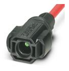
Device connector front mounting, Range of articles: SUNCLIX, housing material: PPE, color: black, number of positions: 1, min. conductor cross section: 2.5 mm<sup>2</sup>, rated voltage: 1000 V DC, rated current: 27 A, Connection method: Crimp, Contact connection type: Pin, cable length: 130
