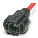
Device connector front mounting, Range of articles: SUNCLIX, housing material: PPE, color: black, number of positions: 1, min. conductor cross section: 6 mm<sup>2</sup>, Connection method: Crimp, Contact connection type: Pin, cable length: 130
