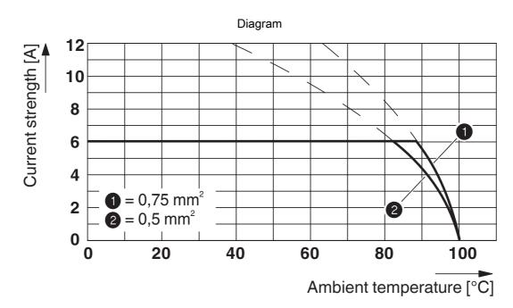
Type: PTSM 0,5/...-2,5-H SMD WH (L) R.. Tested in accordance with DIN EN 60512-5-2:2003-01 Reduction factor = 1 Number of positions: 5
